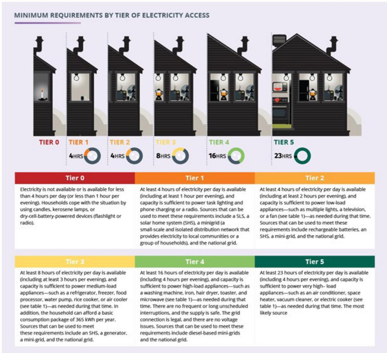
Figure 6 - Electricity Access Levels by ESMAP<sup>9</sup>
